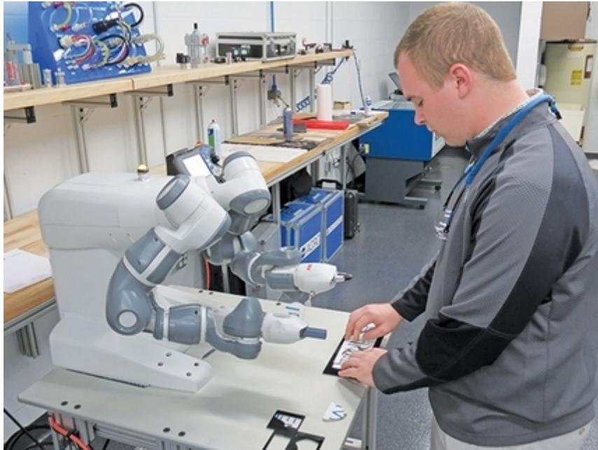
Zach Hoerr, a mechanical engineer with Penn-Air & Hydraulics' automation team, demonstrates how the ABB YuMi dual-arm robot can work with humans on precision manufacturing tasks involving small objects. Hoerr, the company's YuMi specialist, programmed the device to put together a puzzle made up of acrylic pieces as part of a demonstration at Penn-Air's Springettsbury Township headquarters in York County. - (Photo / Roger DuPuis)
