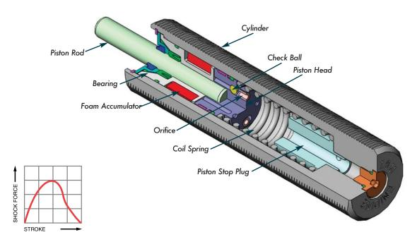
Constant orifice area damping (dashpot) provides the largest shock force at the beginning of the stroke when impact velocity is highest. These shock absorbers provide high-energy absorption in a small, economical design.
